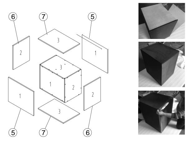
A. Tear off the double-sided adhesive on Foam Sheet 3 (7) and attach Foam Sheet 3 (7) to Board 3.
