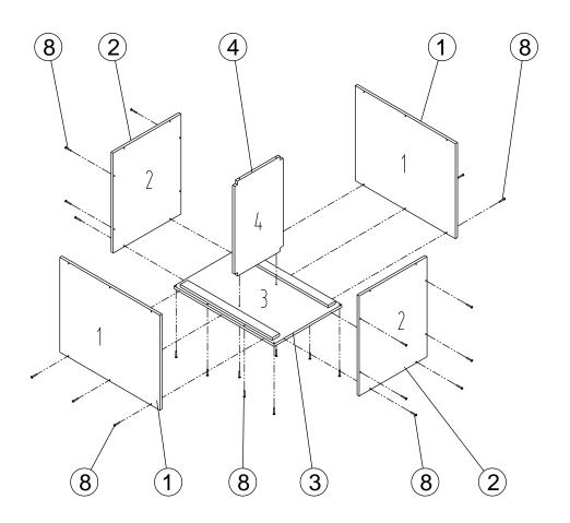
A. Attach two Boards 1 (1) to Board 3 (3) using fourteen Screws (8).
