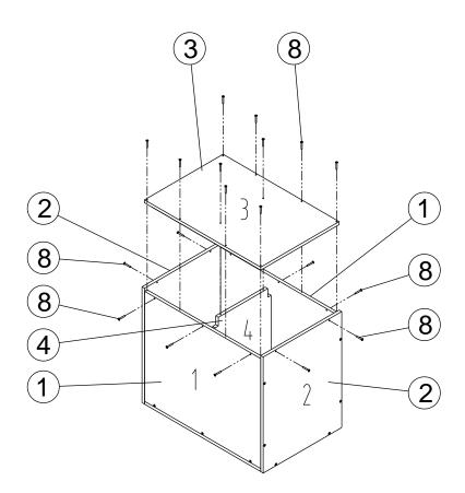
A. Attach another Board 3 (3) to Boards 1, 2, 4 (1,2,4) using twenty Screws (8).
